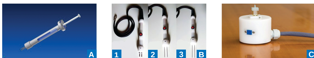
Figure 2. (A) Schematic representation of a syringe for the injection for GET procedure through electric fields; (B) different types of electrodes used for ECT; (1) Reusable and removable electrode plates (steel 3 mm); (2) Reusable and removable two-needle unshielded electrode, steel 40 mm and (3) steel 52 mm; (C) electroporation cuvette inserted in a cuvette holder modified for EP-TVL.
